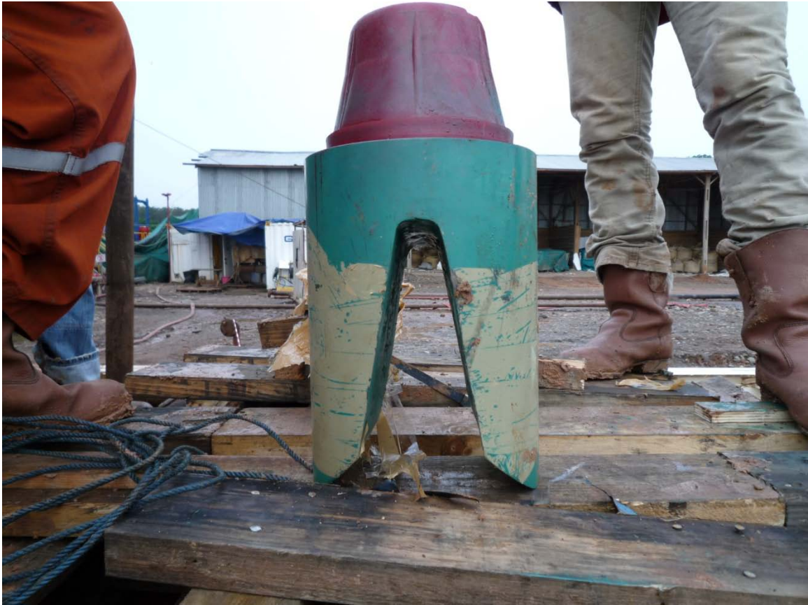
Reverse "screw driver" used to back off the landing joint
