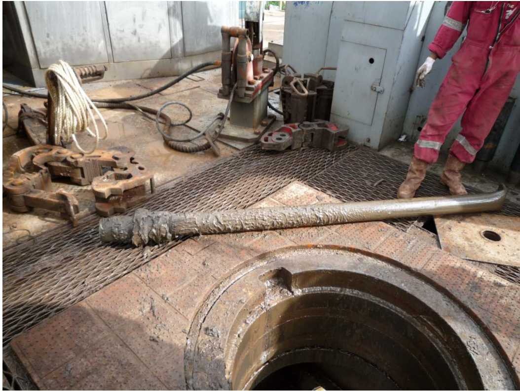
Sheared off lower section of landing joint after recovery
