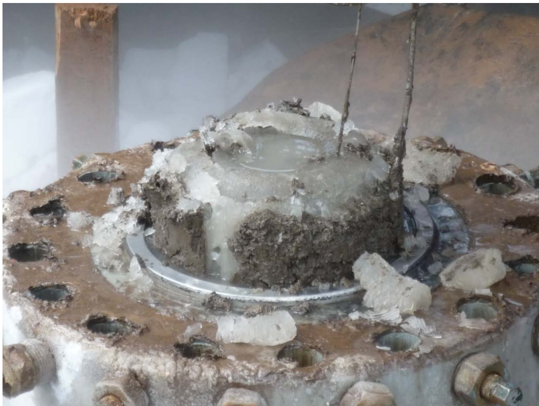
Top of C-Section (tubing hanger) upon lifting off the BOP (Note the 0.092 wire and ice that formed 2 feet above top of dry ice application)
