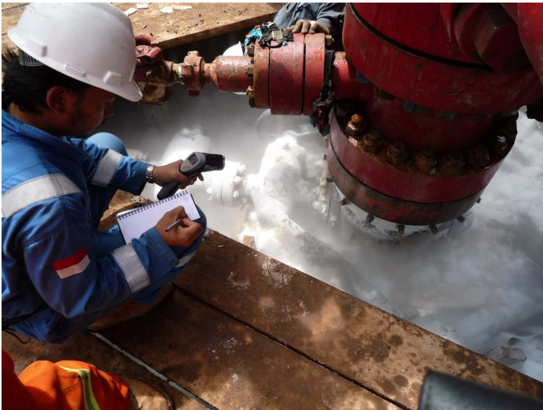
Recording wellhead temperature with handheld device
