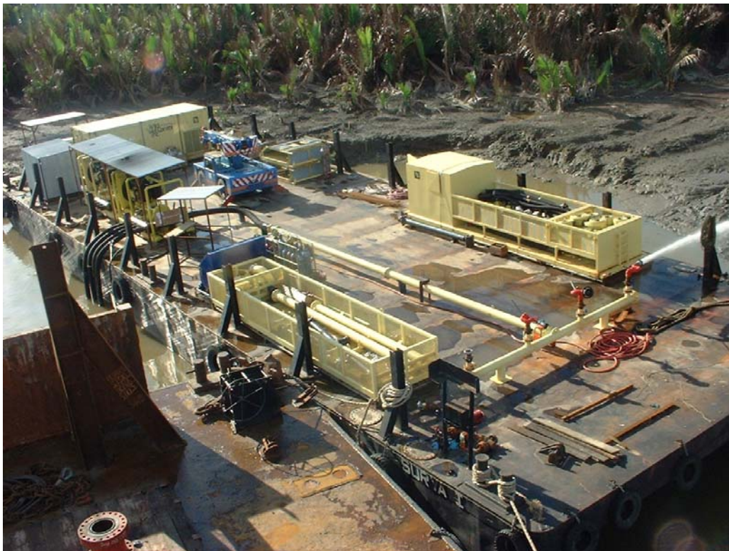
Figure 5.2 Barge Supported Firefighting Spread
